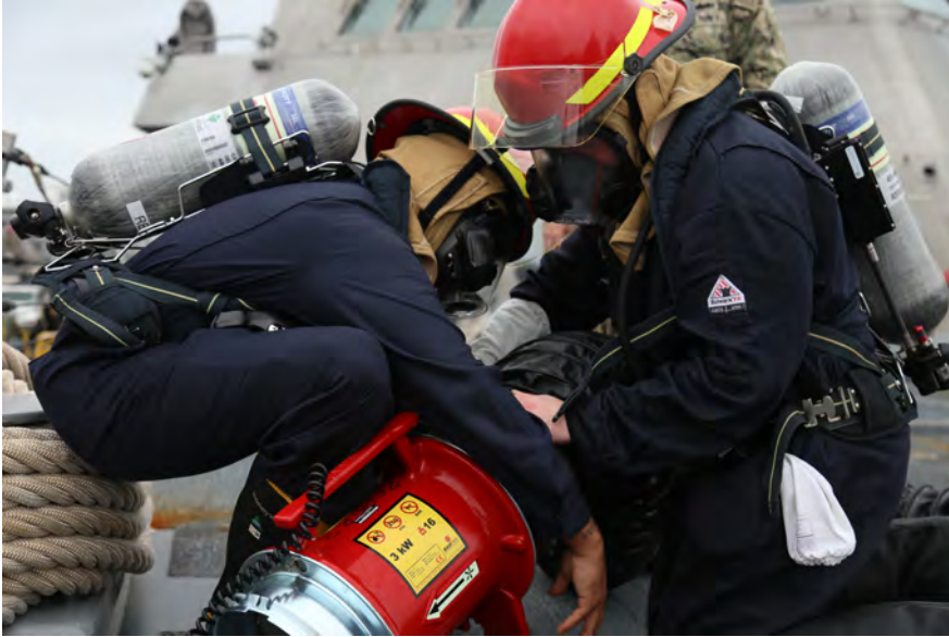
MSP Crewmembers set up a RAM Fan for de-smoking operations onboard LCS-19.
